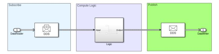
In the Simulink model for the Shapes Demo, view how the DDS blocks, Take DDS Sample and Write DDS Sample, are used to subscribe to and publish the location of the shape.
